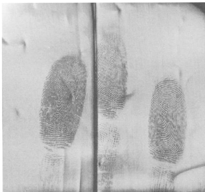
FIG. 3—Cyanoacrylate-treated fingerprints on clear plastic. Field of view is 6\text{ cm} \times 6\text{ cm} . The intensity of the incoming beam from the 5 mW HeNe laser has been reduced by a factor of 1000 using an O.D. 3.0 neutral density filter.
