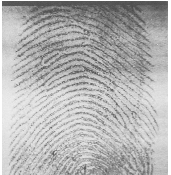
FIG. 6b—Magnified image of part of the fingerprint. Field of view is 1.5 cm × 1.5 cm. 5 mW HeNe laser with O.D. 3.0 ND filter.
