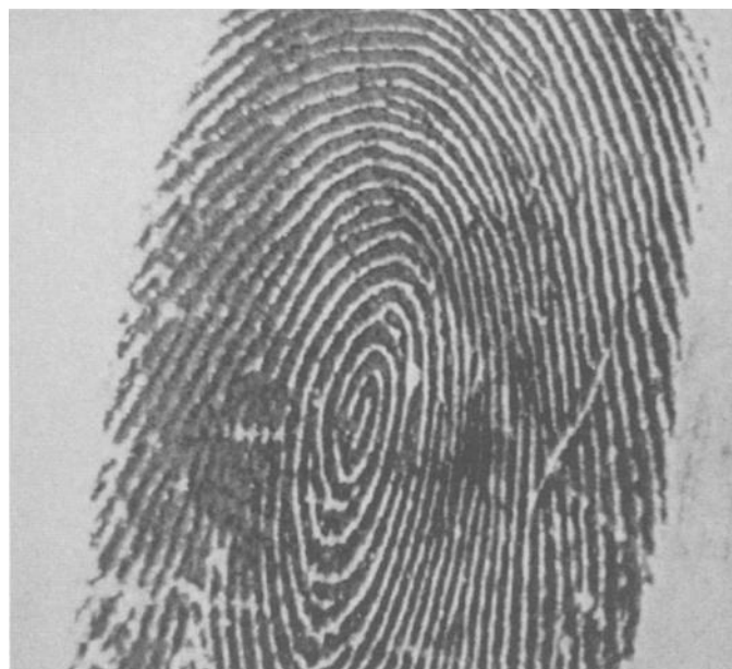
FIG. 4b—Magnified image of part of the above fingerprint. Field of view is 1.5\text{ cm} \times 1.5\text{ cm} . 5 mW HeNe laser with O.D. 3.0 ND filter.
