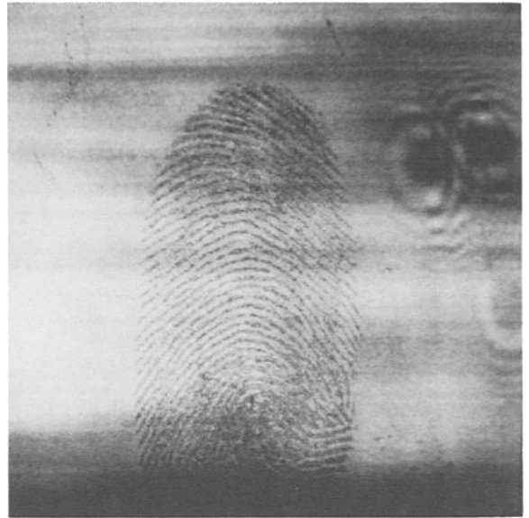
FIG. 6a—Untreated fingerprint on the polished surface of a silicon wafer; entire fingerprint. Field of view is 3 cm × 3 cm.
