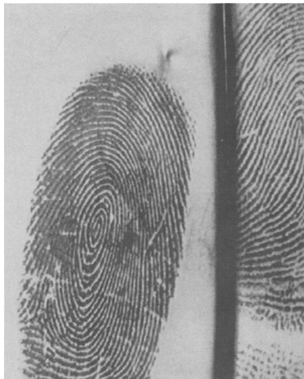
FIG. 4a—Cyanoacrylate-treated fingerprint on clear plastic; entire fingerprint. Field of view is 3\text{ cm} \times 3\text{ cm} .
