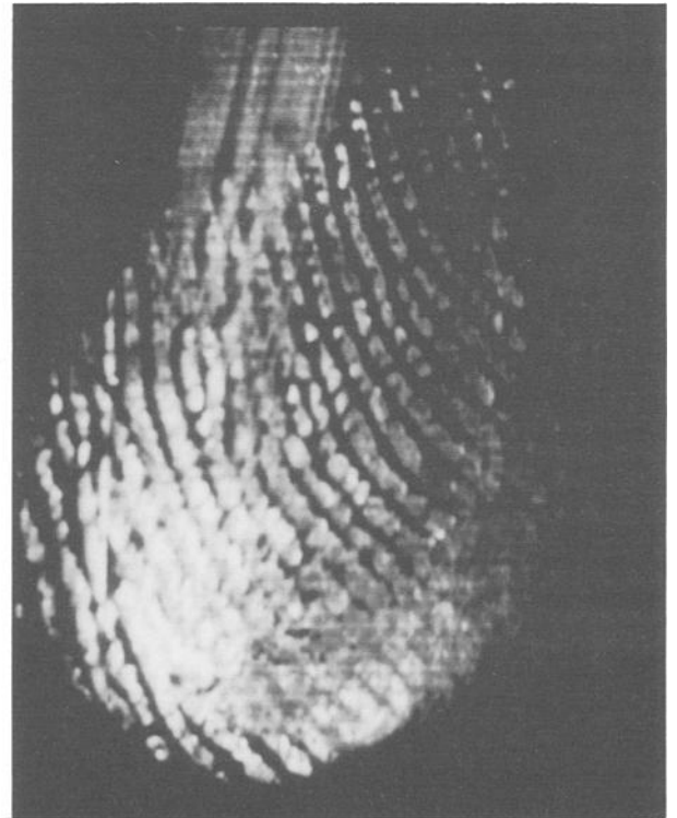
FIG. 8d—Fluorescence image. The laser beam is focused onto the sample surface through the clear plastic. 60 mW ArKr laser plus 10 nm narrow bandpass filter centered at 488 nm. Measured power at 488 nm incident on the sample = 0.5 mW. An O.D. 4.0 ND filter was used in front of the detector for the reflected-light images only.
