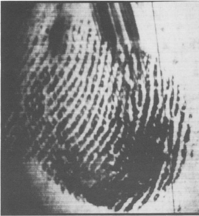
FIG. 8a—Rhodamine-treated fingerprint on clear plastic. Field of view is 3 cm × 3 cm; (a) reflection image. The laser beam is focused onto the sample surface from the fingerprint side.
