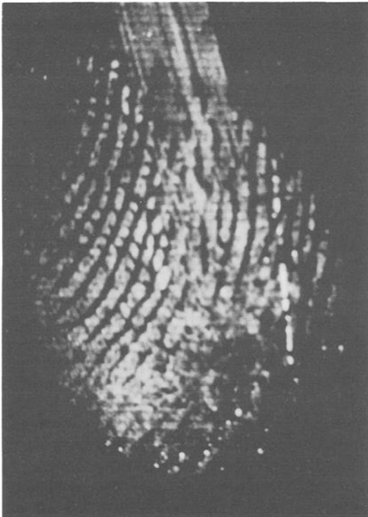
FIG. 8c—Fluorescence image. The laser beam is focused onto the sample surface from the fingerprint side.
